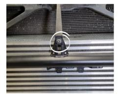
Remove the bushings and brackets from the OEM intercooler and install it on the do88 intercooler in the same positions as mounted on the OEM.
