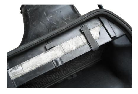
From both intercoolers, remove the intercooler inlet air guide by unclipping the 6 metal fasteners that holds it to the outlet air guide with a flat screw driver
