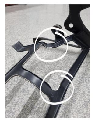
After you have made the cuts the air guides needs to be heated in the marked areas and then pressed against the bottom of the intercooler to mold after each other.
