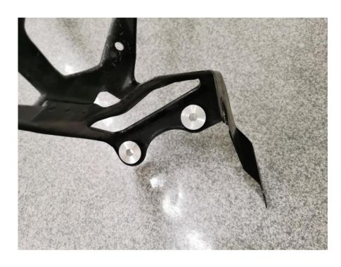
Insert the aluminium bushings in the intercooler support frame, 4pcs a side.
