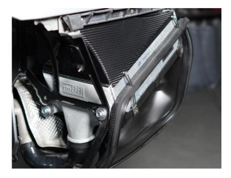
When mounting the intercooler into the support frame start by laying the bottom air guide in place. Then take the intercooler and place it on top and fasten it with the included m8 bolts through the aluminum bushings.
