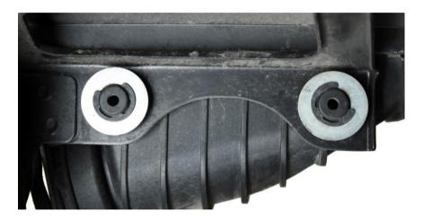
From front part of the intercooler support frame on both sides remove the two 13mm hex screws and one 13mm nut .
