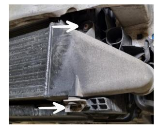
Remove 3x Torx T25 and disconnect the cable clips along the crash bar.
