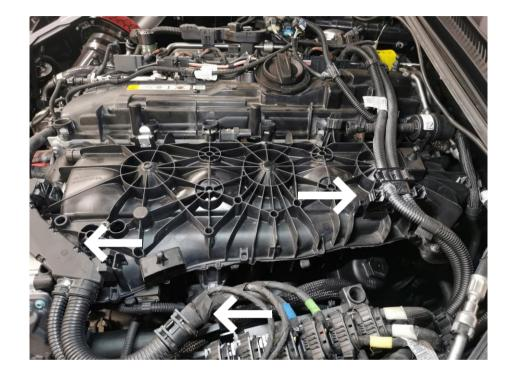
Remove the T20 screw holding the EVAP line to the intake manifold and disconnect the 3 lines and remove them. Disconnect the EVAP valve from the fuel tank breather line and put it to the side.
