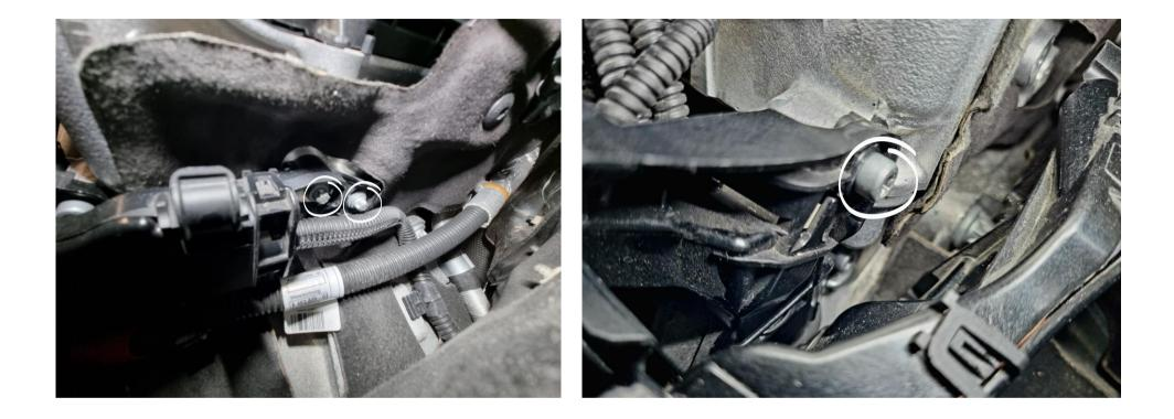
In the rear end of the engine, remove the 2 x E8 screws holding the outer wire harness channel on the back of the engine. Separate outer wire channel from the inner one and move it a bit backwards.
