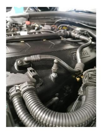
Mount the long engine cover mount to the intake manifold with washers or a nut as height adjustment and the short one to the large bracket in the rear of the manifold.
