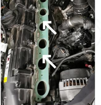
Mount 6pcs of the included sealing rings to the intake manifold flange.
