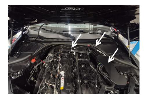
Remove the engine cover and disconnect the electrical connectors from the charge pipe, front water pump and intake air temp sensor on the manifold.
