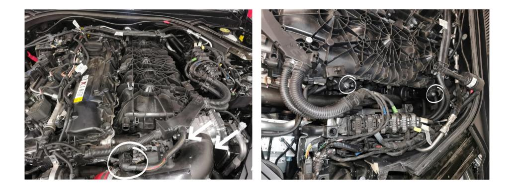
Remove the 2 screws holding the charge pipe to the throttle body, then remove the 3 screws holding the throttle body to the intake manifold. Disconnect the throttle body electrical connector and unclip the harness from the intake manifold.
