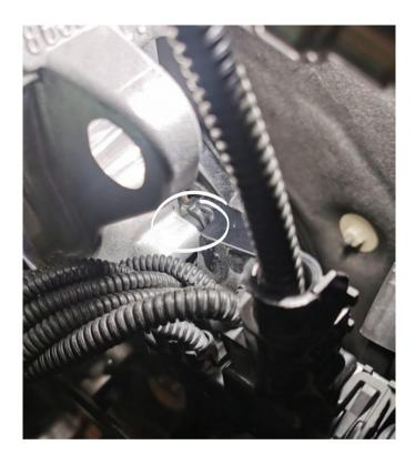
Mount the included plastic spacer between the channel and engine to move it back a bit and reinstall the T30 holding the inner wire channel.
