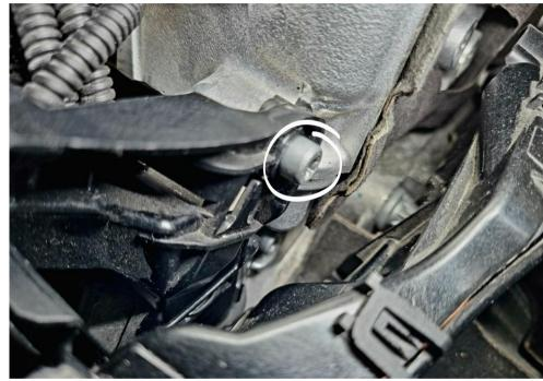
In the rear end of the engine, remove the 2 x E8 screws holding the outer wire harness channel on the back of the engine. Separate outer wire channel from the inner one and move it a bit backwards.
