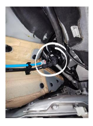
Now mount the short hose side to the connection down in the transmission tunnel and feed the other end up to the engine bay close to the firewall. Then secure it with included zip-tie.
