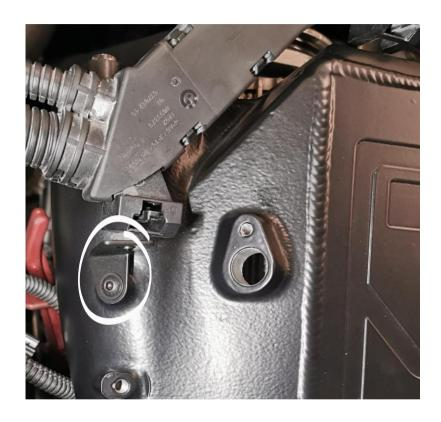
Fasten the rear bracket for the front wiring channel to the intake manifold with 1  $\times$  M5 screw included.
