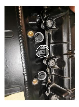
Mount the do88 Performance intake manifold to the cylinder head. Align it over the headless screws and backing them out until they are halfway into the manifold flange.
