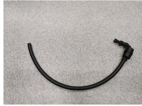
Remove 8 x 8mm hex screws from the underflooring and remove it to reveal the lower EVAP connection (the black plastic line in the transmission tunnel). Disconnect it and remove it upwards.
