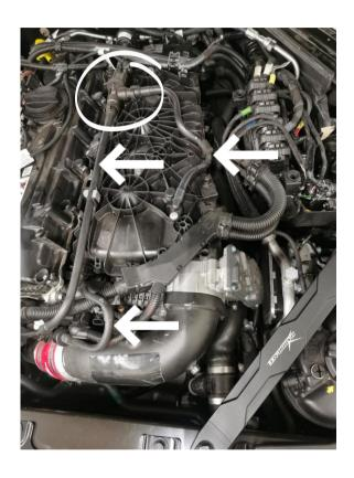
Remove the T20 screw holding the EVAP line to the intake manifold and disconnect the 3 lines and remove them. Disconnect the EVAP valve from the fuel tank breather line and put it to the side.
