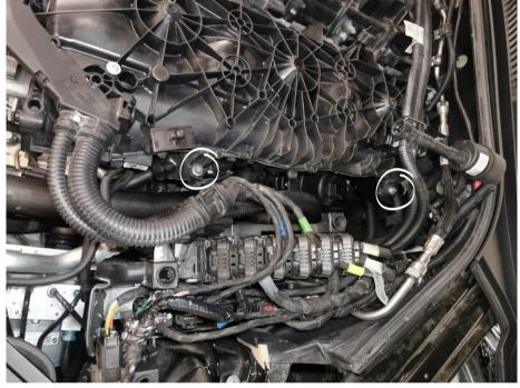
Remove the 2 screws holding the charge pipe to the throttle body, then remove the 3 screws holding the throttle body to the intake manifold. Disconnect the throttle body electrical connector and unclip the harness from the intake manifold.
