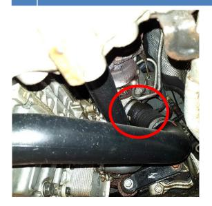
**4.** Remove 3x Hex 10mm screws that holds the plastic intercooler pipe.
