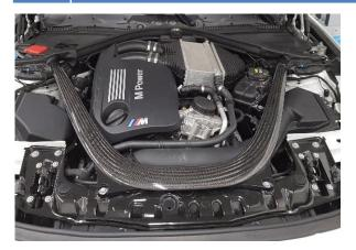
Remove 4x 6mm hose clamp from both intercooler pipe hoses. Slide the hoses on to the intercooler pipes as much as possible.
