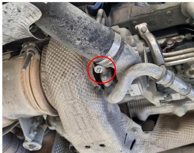
**25.** Remove the intercooler inlet hoses and the BOV hoses from air boxes.
