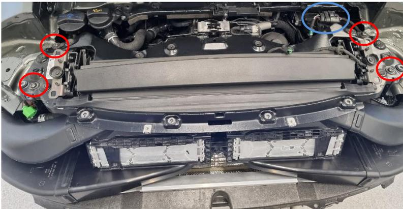
**20.** On both sides remove the two air ducts.
